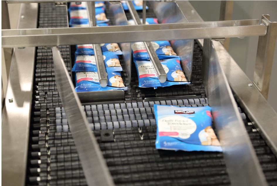
WET WIPES CAN BE MOVING AT VARIABLE SPEEDS ON DIFFERENT SECTIONS OF THE CONVEYOR AS DICTATED BY THROUGHPUT REQUIREMENTS.
