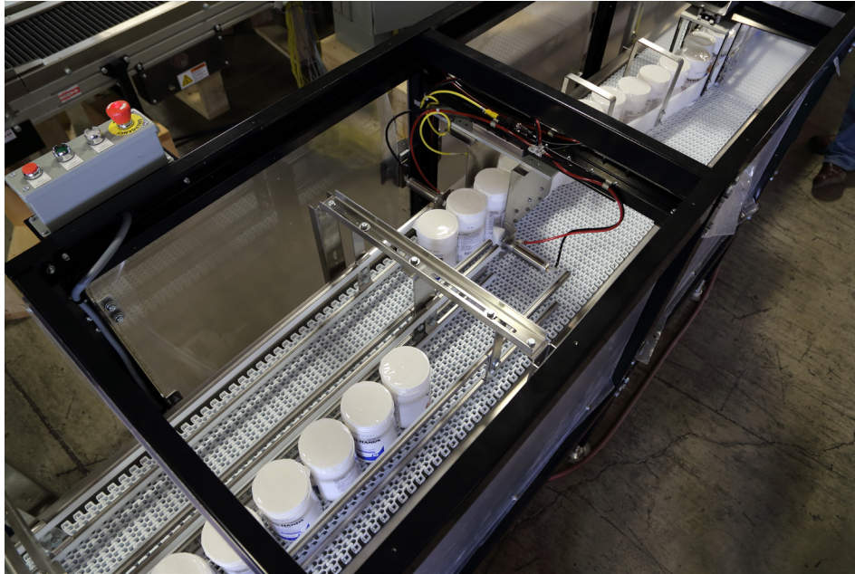
WET WIPES CAN BE MOVED FROM ONE CONVEYOR TRAFFIC LANE TO ANOTHER TRAVELING IN THE SAME OR THE OPPOSITE DIRECTION.
